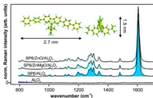
Fig. 1: Raman spectra of 8 nm SP6 on sapphire, ZnMgO(000-1), and ZnO(000-1). The bottom spectrum depicts the sapphire response for comparison. Inset: SP6 molecule as calculated by DFT.
