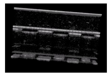
Researchers used entangled photons to increase the penetration depth of OCT for scattering materials. They demonstrated the technique by analyzing two alumina ceramic stacks containing laser-milled microchannels. The mid-infrared illumination allowed the researchers to capture depth information and to create a full 3D reconstruction of the channel structures (pictured).
