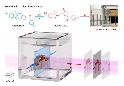
Their invention is based on Hecht's specialty: photoswitchable molecules, which only at the intersection (xolography) of light rays of two different colors allow precise curing of the starting material in the entire volume (holos). In combination with a new printing process (xolography) based on a laser-generated light sheet and projected cross-sectional images, the desired objects are generated from virtual 3D models.
