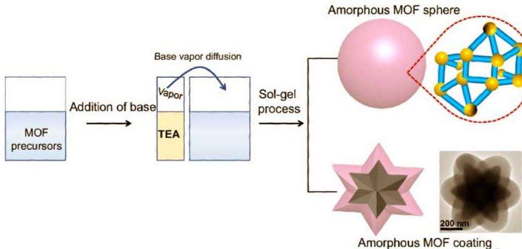
The synthesis of aMOFs and aCPs colloids and core-shell structures via mimicking the Stober method.
