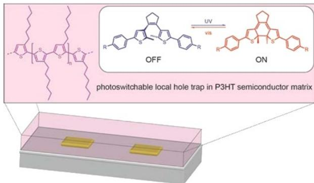
Figure: “Smart” transistors gated by light: UV-illumination transforms ring-open dithienylethene (blue) to its ring-closed isomer (red), which effectively traps holes in the semiconducting poly(3-hexylthiophene) (P3HT) matrix. Illumination with visible light reverts the process and reinstalls charge flow through the device.
